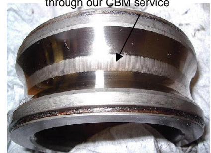
Bearing Flutting detected through our CBM service
